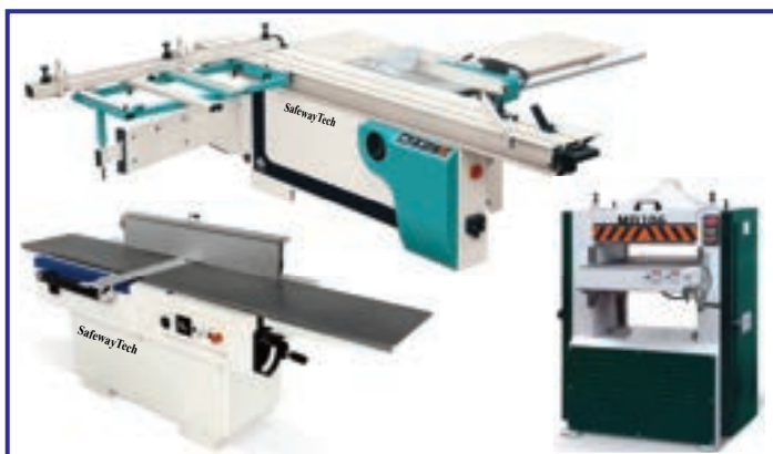
Thickneture, Jointer & Saw Machine
