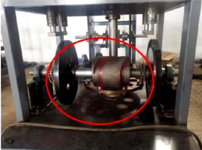
open cam system instead of gear box
